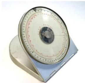
The original ALRO calculating disc is famous for its patented assembly of fixed and moving circular parts, housed in a hinged collapsible box that was used for protection when closed; but also - when unfolded - it provided an optimal “hands-free” desk stand.
